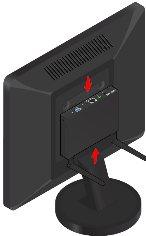
Figure 34: Connecting the cables to the VIA ARTiGO A920
