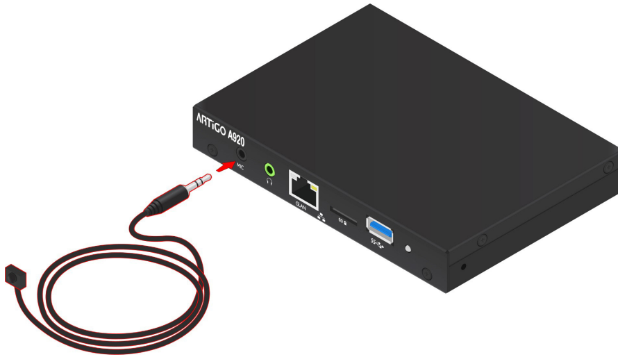
Figure 29: Connecting the Consumer Infrared (CIR) receiver cable
